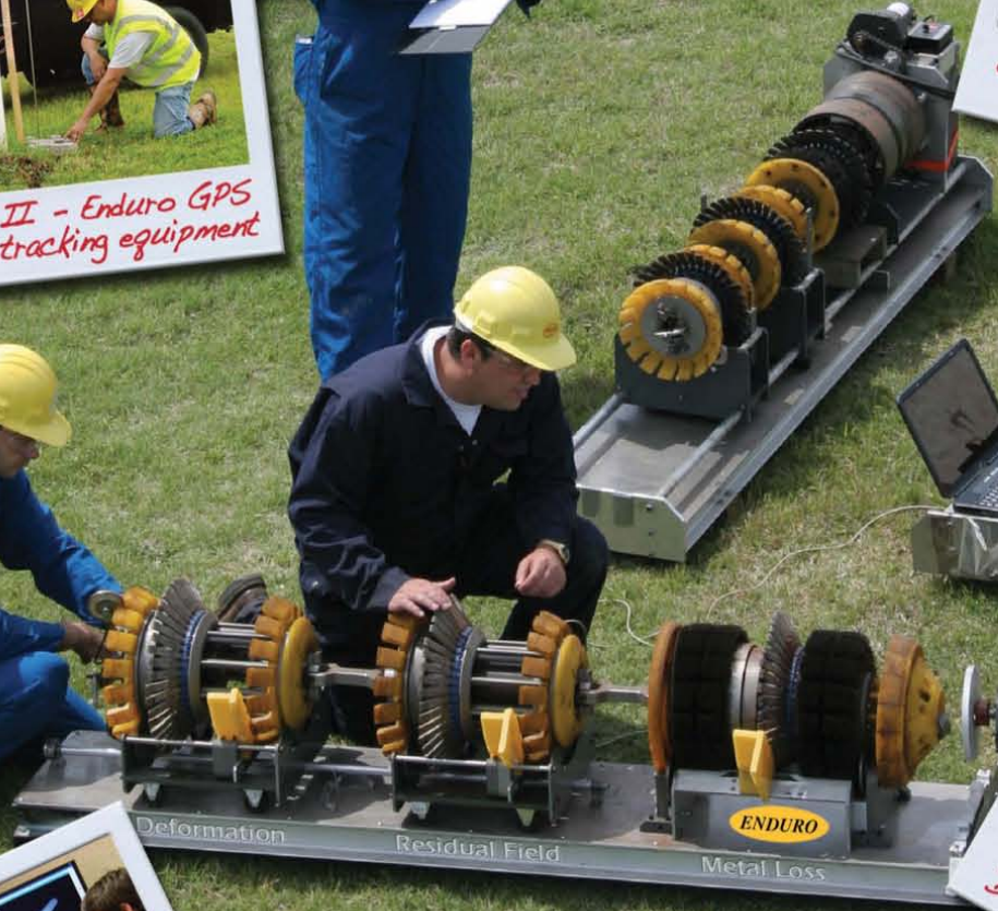
Stage I - Enduro Cleaning pig train
