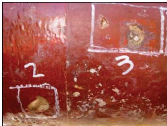
The acidic soil environment created by the coal seam, moisture, and elevated temperatures caused the coating disbondment and external pitting corrosion shown here, despite cathodic protection (Fig. 4).
