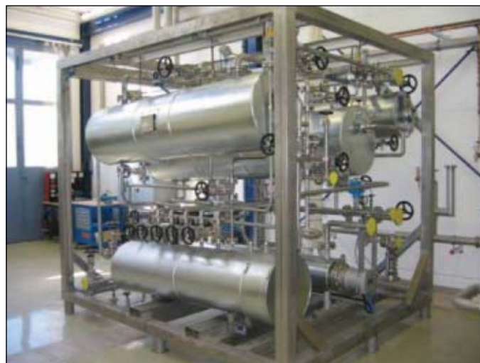
This custom-made cryocondensation unit has a gas capacity throughput about 100 std. m cu/hr and cooling power of about 100 kw (Fig. 5).
