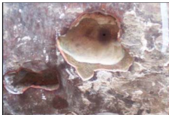
The acidic soil environment created by the coal seam, moisture, and elevated temperatures caused the coating disbondment and external pitting corrosion shown here, despite cathodic protection (Fig. 4).
